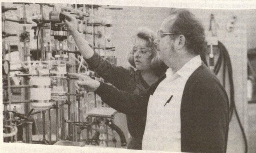
Chemistry Laboratory: High-vacuum lab for study of kinetics of decompositions of organosilanes and silicon hydrides.
